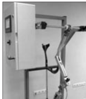
Fig. 2. A photograph of the newly designed artificial arm with elbow joint
