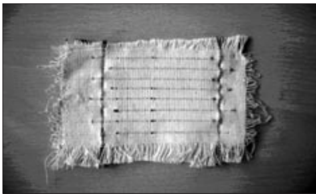
Fig. 1. Woven sample with stainless steel yarns
