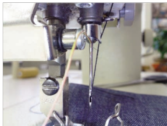
Fig. 2. Placement of thermocouple inside the needle groove
