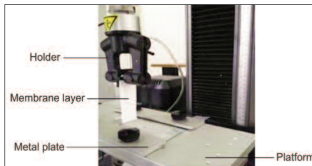
Fig. 2. Schematic diagram of electronic universal-testing machine
