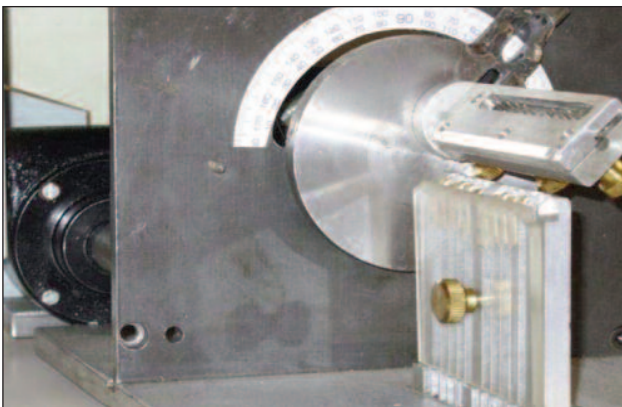
Fig. 1. The prototype device to measure resistance to bending
