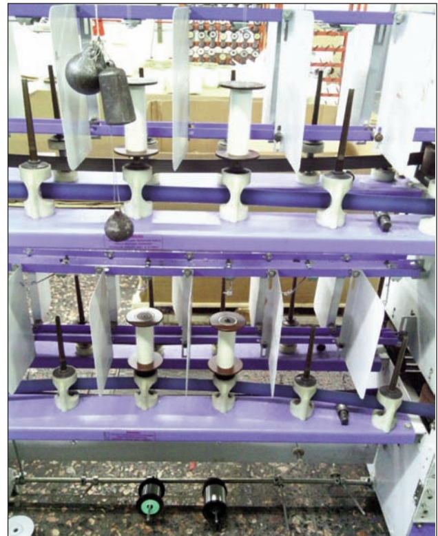
Fig. 3. Photo of the hollow spindle twisting machine (MX model, Sapru Machines Pvt.Ltd)
