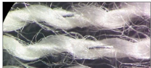
Fig. 4. Stereomicroscopic Images (20×) of the a) C_{11} coded composite yarns (Double layer SS/PP wrapped yarns made with 50 \mu\text{m} SS) and b) C_{32} coded composite yarns (Double layer SS/ PES-Cotton Core-spun wrapped yarns)
