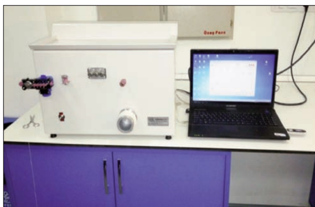
Fig. 5. Photo of the coefficient of friction measurement device (Duranax-E.F.I.)
