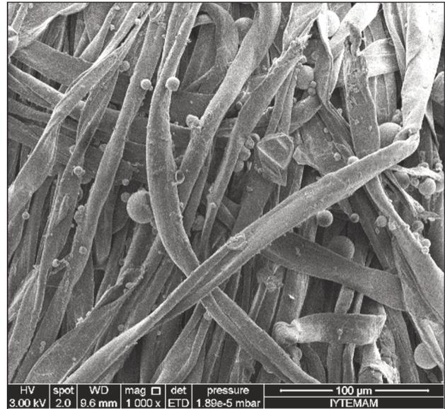
Fig. 4. SEM images of 8 g/L microcapsule, 1.8 g/L binder (left) and 2.5 g/L binder (right) applied fabrics with a magnification of (1000 x)
