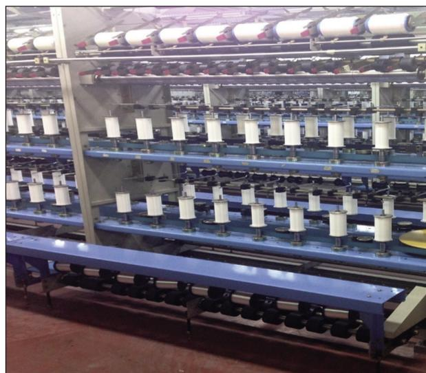
Fig. 1. Hollow spindle spinning machine
