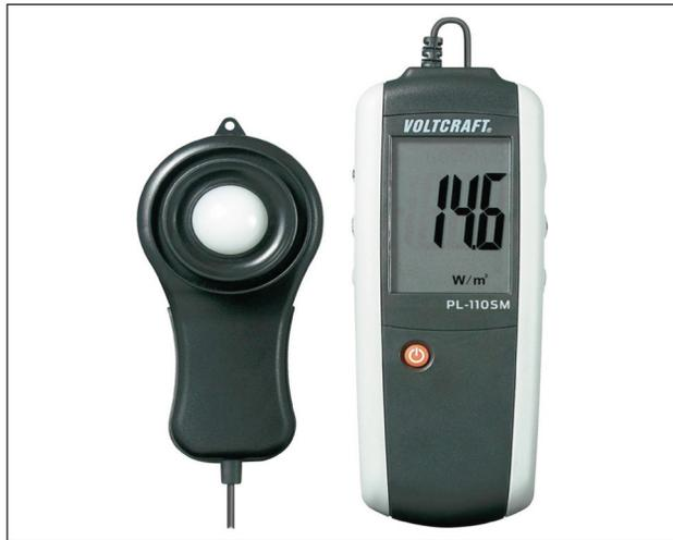
Fig. 3. Voltcraft PL-110SM Pyranometer [17]
