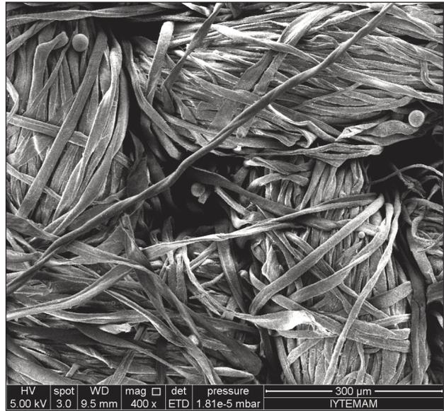
Fig. 2. SEM images of 4 g/L microcapsule, 1.8 g/L binder (left, 1000 x) and 2.5 g/L binder (right, 400 x) applied fabrics
