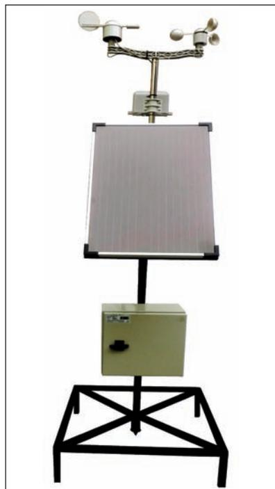
Fig. 6. The meteorological stations
