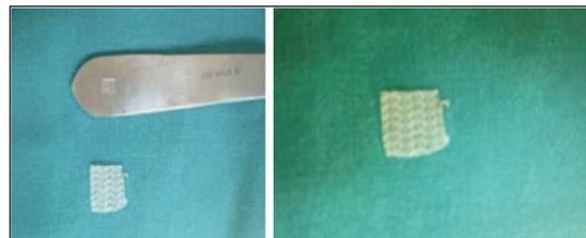
Fig. 4. Collagen-coated polypropylene mesh
