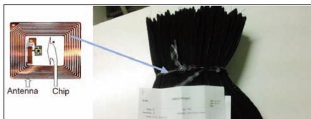
Fig. 3. Batch with RFID tag
