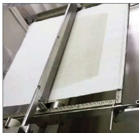
Fig. 1. Thin-film based on metal microparticle deposition using laboratory coating device type SV
