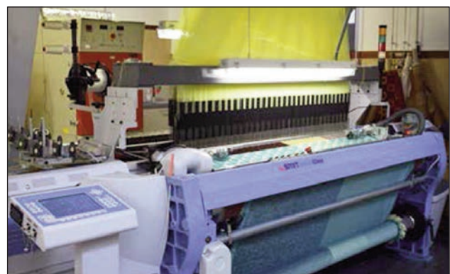
Fig. 2. The fabric made by Smit Textile GS900 Jacquard Loom
