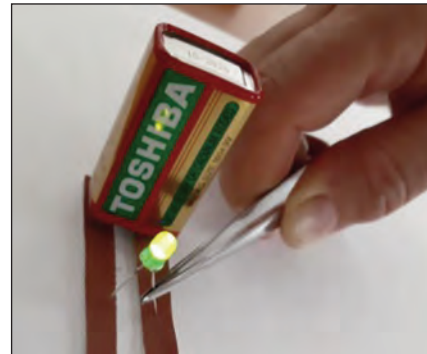
Fig. 2. Electrical conductivity test for sample 10
