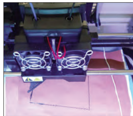
Fig. 3. 3D printing on the surface coated with paste based Cu microparticles
