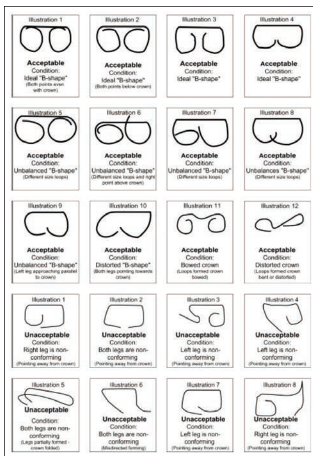
Fig. 1. Acceptable and unacceptable forms of the staple line [3]
