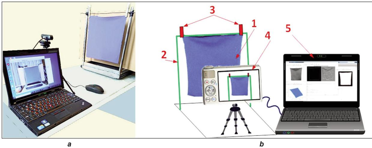
Fig. 1. Experimental set-up for obtaining drape images: a – general view; b – principle schematic
