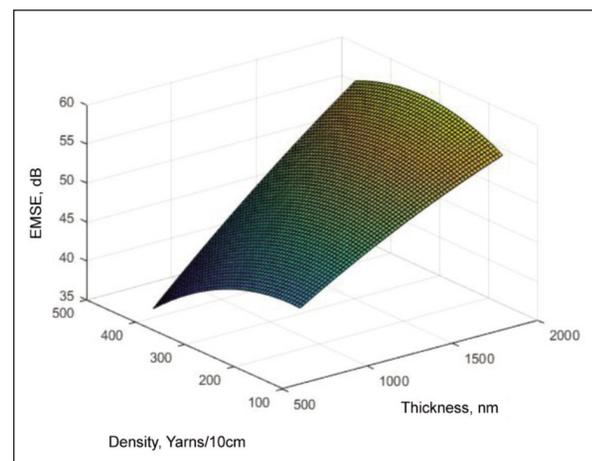
Fig. 5. MATLAB plot of the EMSE response surface
