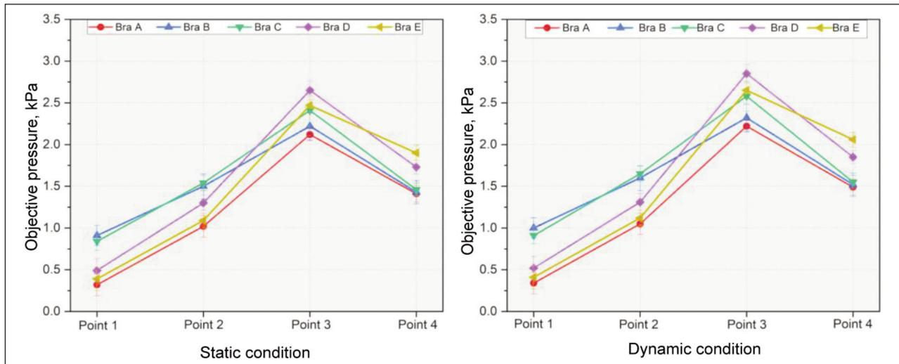
Fig. 3. The pressure distribution of 5 seamless sports bras
